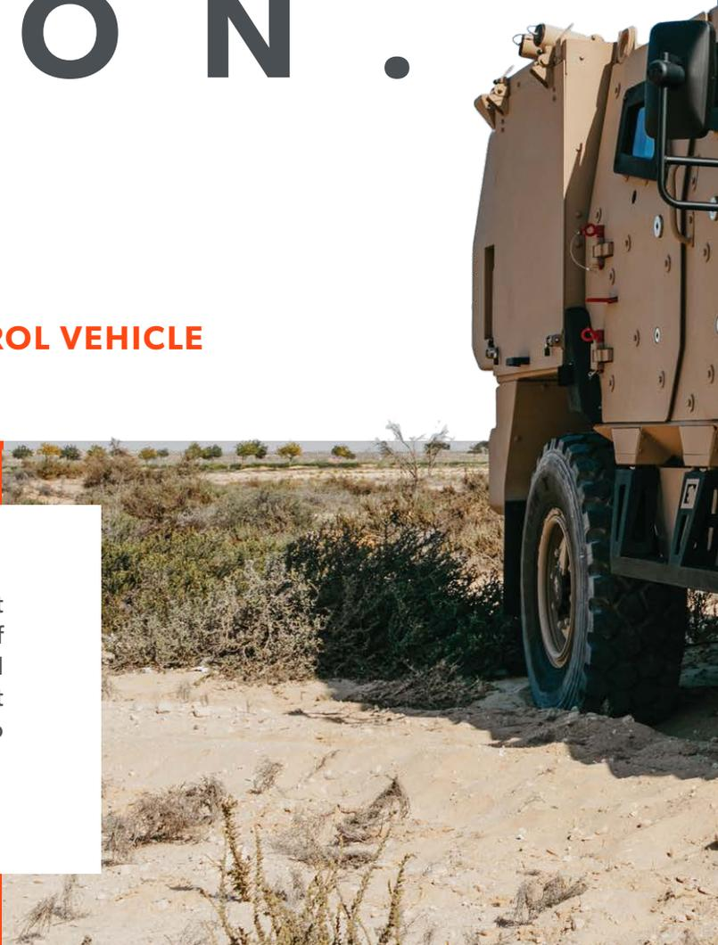
Capable of accommodating a roof-mounted self-defence weapon, the vehicle also has full-time four-wheel drive powered by a diesel, water-cooled turbocharged engine. A central tyre inflation system (CTIS) allows tyres to be inflated or deflated to meet terrain conditions.
