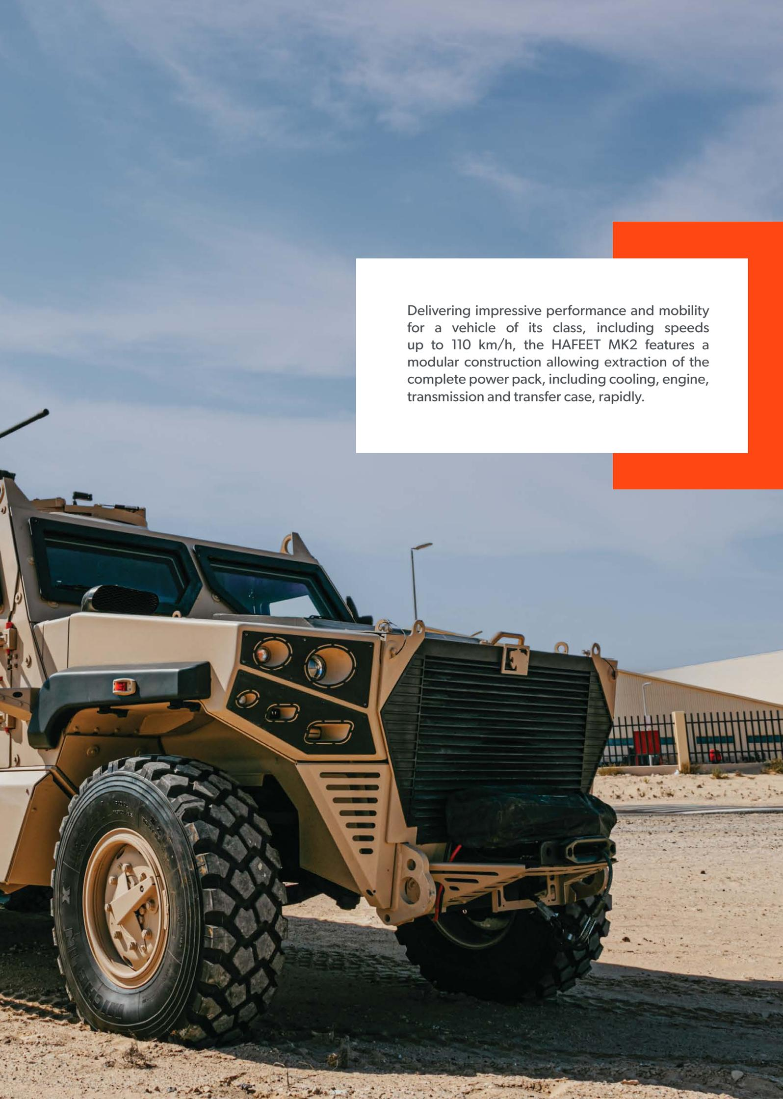
Delivering impressive performance and mobility for a vehicle of its class, including speeds up to 110 km/h, the HAFEET MK2 features a modular construction allowing extraction of the complete power pack, including cooling, engine, transmission and transfer case, rapidly.
