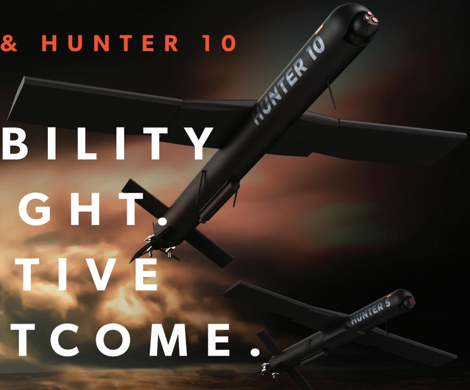
The HUNTER 5 and 10 possess a take-off weight of 50 kg and can be fired from the back of an armored vehicle. It carries a payload of 5 kg and 10 Kg, respectively. The drones flies at a maximum altitude of 7000 ft. The drones are suitable for recon and attack missions, operating at a cruising speed of 120km/hr, with endurance of 180 minutes for HUNTER 5 and 150 minutes for HUNTER 10. It features a wing span of 3.6 m, length of 2.85 m and run by a gasoline engine.
