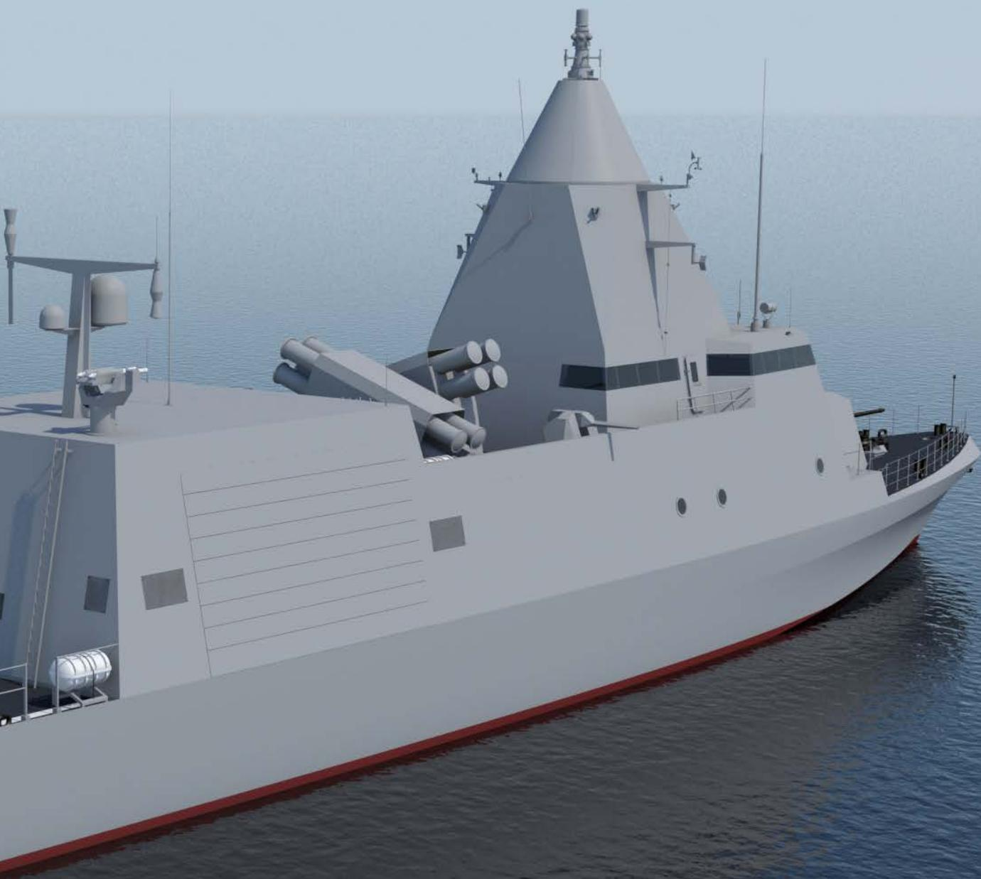
A reduced RCS (radar cross section) and optimised wheelhouse arrangement with wide visibility ensure the MK II is ready for all coastal patrol and surveillance, mine detection, helicopter operations, maritime interdiction, and friendly forces support operations. The platform also carries multidimensional anti-air and anti-surface capabilities.
