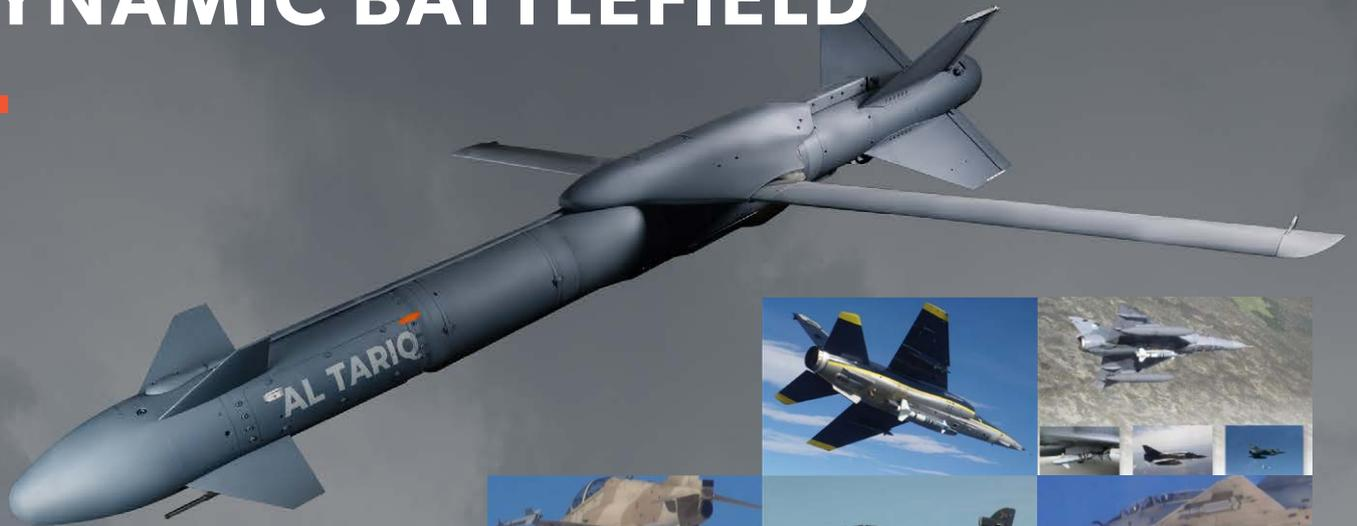
Modular family of Precision Guided kits for the 120/250/450 kg series of aerial bombs. Designed to fulfil operational needs for high accuracy, long stand-off range engagements against stationary, moving and re-locatable targets in a GPS denied environment.
